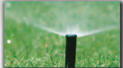
"Pop up" type heads are the most efficient means of watering your lawn. Very little water is placed off target.
